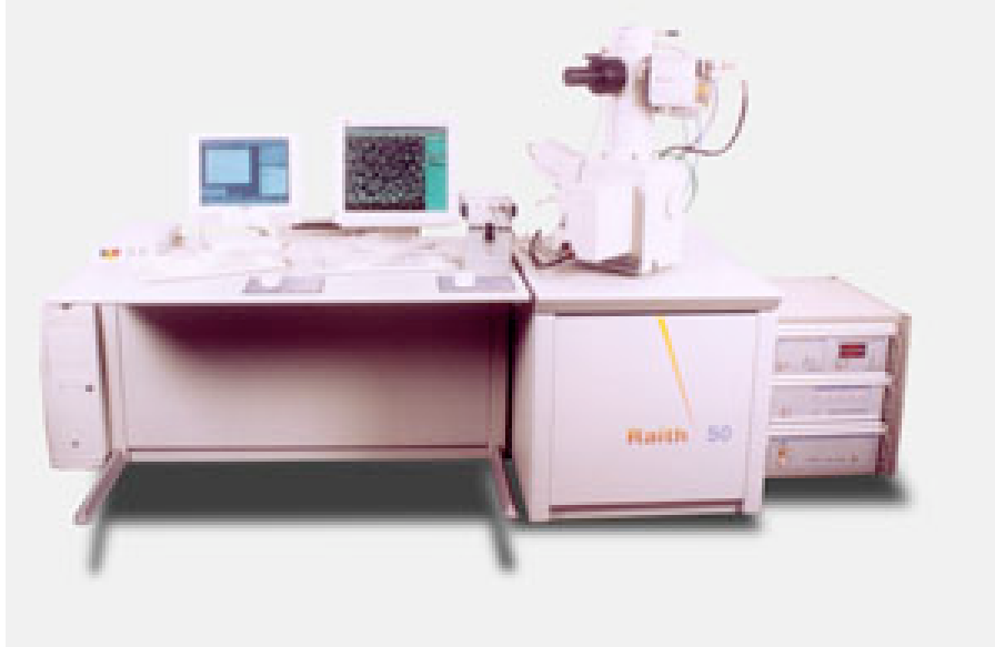
FIGURE 3.11 Raith-50 Electron beam lithography system, picture from the Center for Nano- and Molecular Science and Technology at the University of Texas at Austin.
